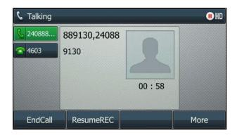
Press the **ResumeREC** soft key again to continue recording. The **III** icon displaying on the status bar changes to **( )** .
