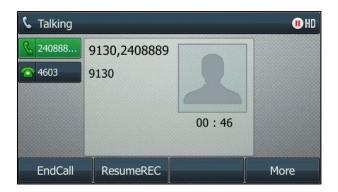
Press the **ResumeREC** soft key again to continue recording. The **11** icon displaying on the status bar changes to **6** .
