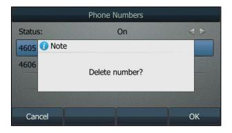
**5.** Press the **OK** soft key to confirm the deleting.
