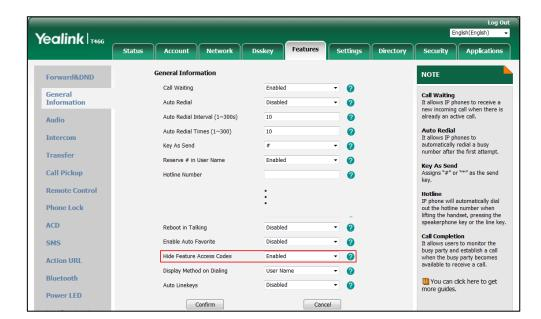
2. Select Enabled from the drop-down menu of Hide Feature Access Codes.
