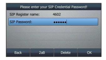
Enter a valid password of the desired SIP account and then press the **OK** soft key to trigger the next authentication. The new password will be saved to the IP phone and override the old password.
