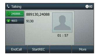
Re-press the **StartREC** soft key to begin a new recording. The recording is saved to a new file on the server.
