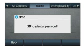
It indicates that the configured SIP password is not valid. The error message will disappear in 2 seconds and the LCD screen will prompt for a password:
