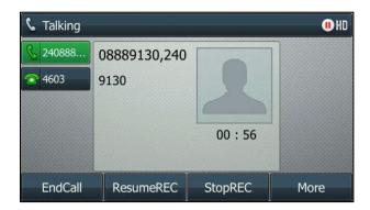
Press the **ResumeREC** soft key again to continue recording. The **!!** icon displaying on the status bar changes to **..**
